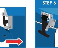
Insert zip-tie through one of the holes on the metal latch hardware.
