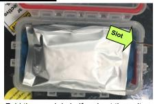
Fold the pouch in half and put the unit back into the protective box. Ensure that the cable is inserted into the slot to prevent cable pinching
