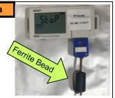
Follow the Data Station instruction to download temperature data, if desired. The data logger may be detached from the thermocouple to move to a remote computer to download data. Once completed go to step 5b
