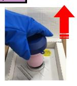
Remove the dry shipper vapor plug.
