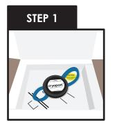
After opening the loaded shipment, ensure the blue Safepak<sup>®</sup> straps stay outside the opening of the dewar at all times.
