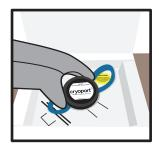
Once the LN2 has been replenished, replace the shipper vapor plug by aligning the slot with the thermocouple wire and gently push the plug into position.
