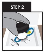
Wearing safety goggles and cryogenic gloves, pull gently upward to remove the shipper vapor plug.
