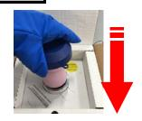
Replace the shipper vapor plug by aligning the slot with the thermocouple wire and gently push the plug into position.
