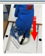
Replace shipper plug. Shipper plug can help insert Tyvek bag into storage well.
