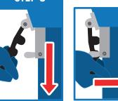
Latch handle on both sides by pulling the black handle down & then towards the shipper.
