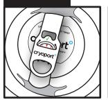
Place the smaller circle handle under the other strap and pull the handle through the slit.
