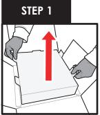
Remove top accessory tray to load commodity. Lift upwards on the white tabs.
