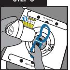
Wear Safety Gloves. Hold the shipper plug in one hand. Hold the blue Safepak® straps with other hand. Pull the shipper plug upwards and out.
