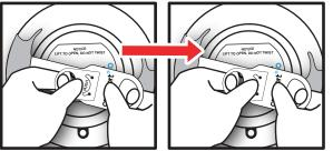
Place your thumb on the word "PUSH" and pull the straps away from each other to place the tab with the word PUSH under the tab with the green check mark.
