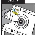
WARNING! Do not leave any samples inside of the shipper. Replace the shipper plug. Push the plug fully into place.
