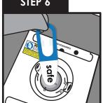
Put the shipper plug to aside. Gently pull upwards on the blue Safepak® straps. Remove sample bag completely and place on a flat surface.
