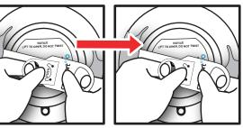
Place your thumb on the word "PUSH" and pull the straps away from each other to place the tab with the word PUSH under the tab with the green check mark.
