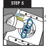
Once the LN2 has been replenished, replace the shipper vapor plug.
