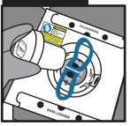
Wearing safety googles and cryogenic gloves, pull gently upward to remove the shipper vapor plug.
