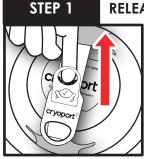
Once the white carton is open, you will need to release the retention band on the shipper plug. Pull the small circle handle up to release the locking tab.
