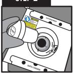
Wearing safety googles and cryogenic gloves, pull gently upward to remove the shipper vapor plug.
