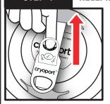
Once the white carton is open, you will need to release the retention band on the shipper plug. Pull the small circle handle up to release the locking tab.
