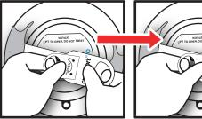
Place your thumb on the word "PUSH" and pull the straps away from each other to place the tab with the word PUSH under the tab with the green check mark.
