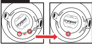
Ensure the hole on the shipper plug and the gray hole on the dewar are aligned. Turn shipper plug to align, if necessary. Also ensure the retention band handles are not overlapping the holes.
