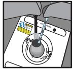
Safely place the cane with the secured goblets or vials and sleeve into the canister and lower into the dewar.
