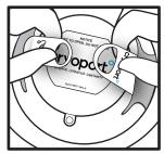
Once the white carton is open, you will need to release the retention band on the shipper plug. Pull the small circle handle up to release the locking tab. Next, unlatch and pull apart the straps.
