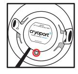
Ensure the hole on the shipper plug and the gray hole on the dewar are aligned. Turn shipper plug to align, if necessary. Also ensure the retention band handles are not overlapping the holes.
