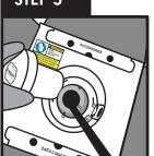
Replace the shipper plug. Make sure the black strap is left on outside of the shipper plug.
