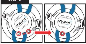
The blue Safepak® straps must be left on the outside of the shipper. Ensure the hole on the shipper plug & the gray hole on the dewar are aligned. Turn shipper plug to align, if necessary. Also ensure the retention band handles are not overlapping the holes.
