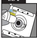
Wearing safety gloves, remove the shipper plug. **CAUTION: Vapors can** escape from chamber during loading.
