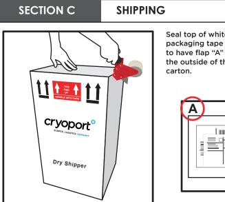
Seal top of white carton with packaging tape making sure to have flap "A" showing on the outside of the white
