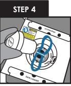
Replace the shipper plug. Shipper plug can be used to help gently insert Safepak® bag down into storage well.
