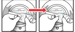
Place your thumb on the word "PUSH" and pull the straps away from each other to place the tab with the word PUSH under the tab with the green check mark.
