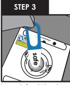
Lower Safepak® bag into shipper and gently push down with gloved hand if necessary.
