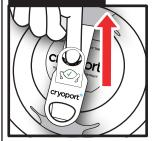
Once the white carton is open, you will need to release the retention band on the shipper plug. Pull the small circle handle up to release the locking tab.
