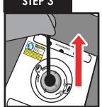
Place the shipper plug to the side. When the commodity is ready to be relocated to another cryogenic storage tank, pull up on the black strap.
