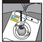
If the straw/commodity is loaded in a goblet or vial on a cane, pull up on the black strap to expose the top of the canister and remove the cane.
