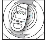
Ensure the PUSH tab is behind the green check mark tab.
