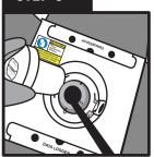
Replace the Lifter or Canister back into the dewar to be returned to **Cryoport.** Replace the shipper plug. Push plug fully into place.
