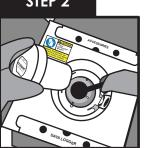
Wear Safety Gloves. While holding on to the black strap, remove the shipper plug. Pull shipper plug upwards and out.
