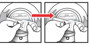
Place your thumb on the word "PUSH" and pull the straps away from each other to place the tab with the word PUSH under the tab with the green check mark.
