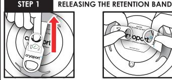
Once the white carton is open, you will need to release the retention band on the shipper plug. Pull the small circle handle up to release the locking tab.
