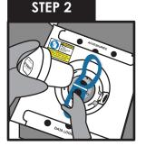
Wear Safety Gloves. Hold the shipper plug in one hand. Hold the blue Safepak<sup>®</sup> straps with other hand. Pull the shipper plug upwards and out.
