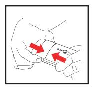
Reattach Control Module to Charge Battery Pack.
