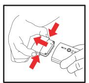
Detach Control Module and attach it to a Mini-USB Charger for 6 hours.
