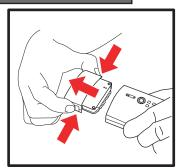
Detach Control Module and reattach it to the a fresh Battery Pack to the new battery pack.
