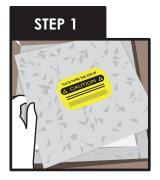
Open box using PPE for cold temperatures and remove the cooler lid. When opening box, be sure not to puncture the shipper. Puncturing the shipper will affect the hold time.
