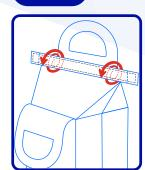
Roll the sealed top down the bag until it reaches the top of the payload.
